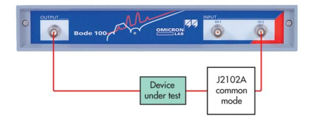
2. When the regulator has a low output voltage, its output can be connected directly to the VNA. When output voltages surpass 3.3 V, the VNA must be capacitively coupled to the regulator.
