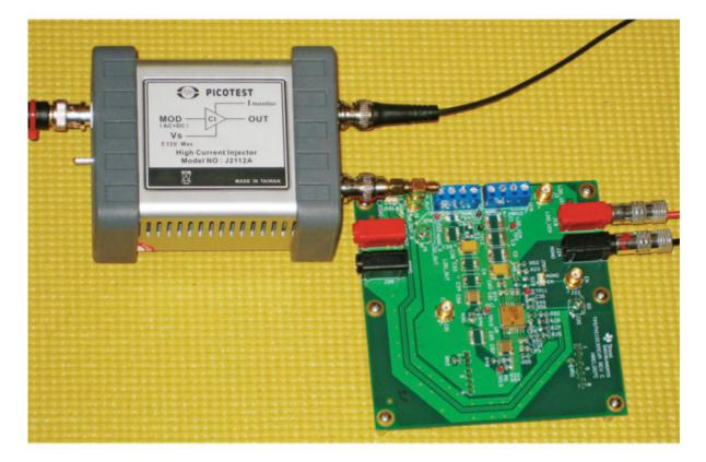
6. A short SMA Tee adapter provides a low-impedance connection between the Texas Instruments demo board and the Picotest J2112A current injector. The J2112A offers very high impedance compared to the regulator and is fast enough not to limit the measurement response.
