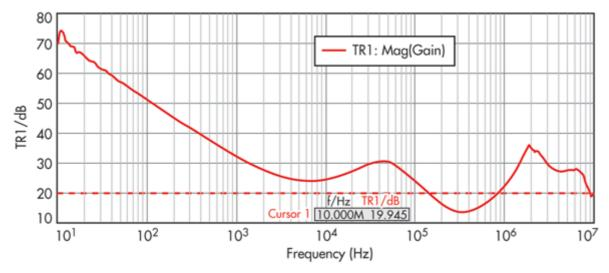
4. The non-invasive stability measurement is made directly at the output of the regulator via the output impedance. The Bode 100 includes proprietary software to convert the measurement directly to a phase margin number.
