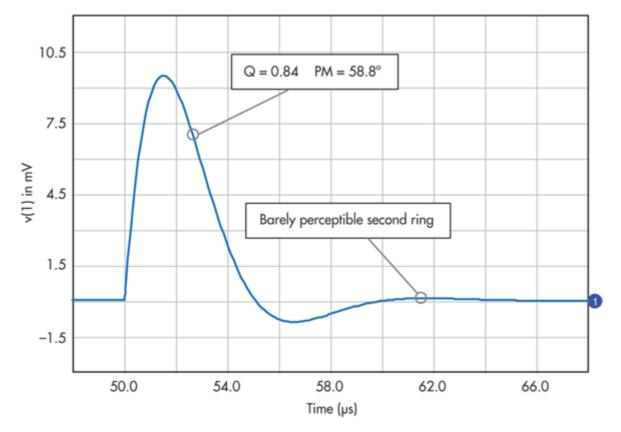
5. The damped transient response corresponds to a 58.8° phase margin, as reported by the Bode 100 non-invasive cursor measurement. Note the barely perceptible second ring.
