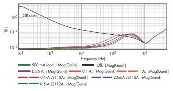
3. The regulator output impedance varies with different load currents and with the regulator unpowered. The bandwidth is approximately 300 kHz, which is evident from the closed-loop magnitude (on state) being greater than the open-loop magnitude (off state) in this region.
