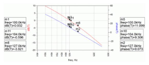
We can equate the stability to an equivalent phase margin by assuming the magnitude of the gain vector to be 1 and solving for the Q.
