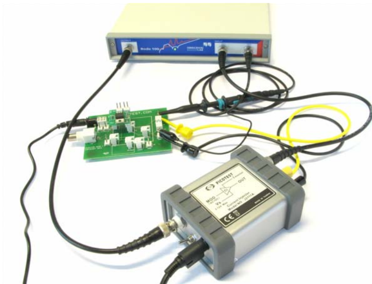
Figure 3: Image showing the Picotest J2111A Current Injector and OMICRON Lab Bode 100 VNA connected to the regulator under test. iv
