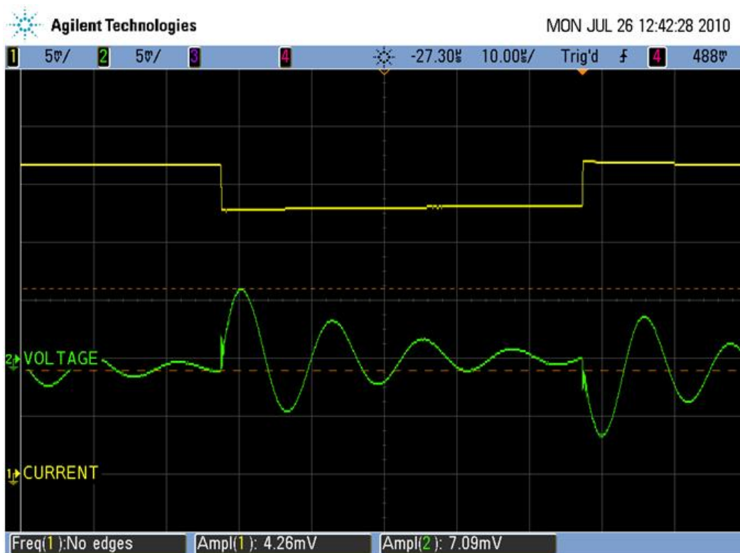
Figure 3. Measured small-signal step-load response (4 mA step) of an LM317T-based regulator circuit with 3.3-V output, 6.3-V input, and a 1- \mu F capacitor.
