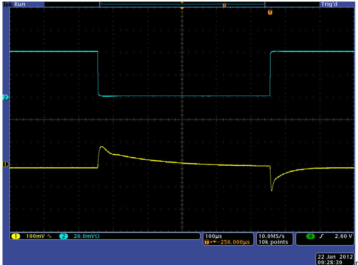
Figure 9 Dynamic load response of 5V output. Blue trace is current (20mA/Div) and yellow trace is voltage (100mV/Div).
