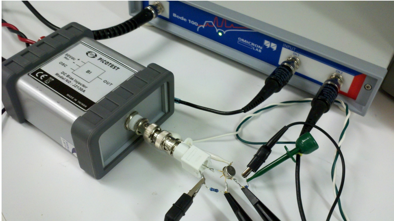
Figure 2 – Photo showing the optocoupler (center) mounted for the measurement.
