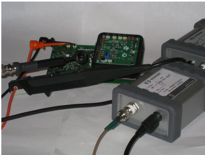
Figure 2 showing the current probe, J2180A preamp and near-field probe with the wireless transmitter/receiver set.
