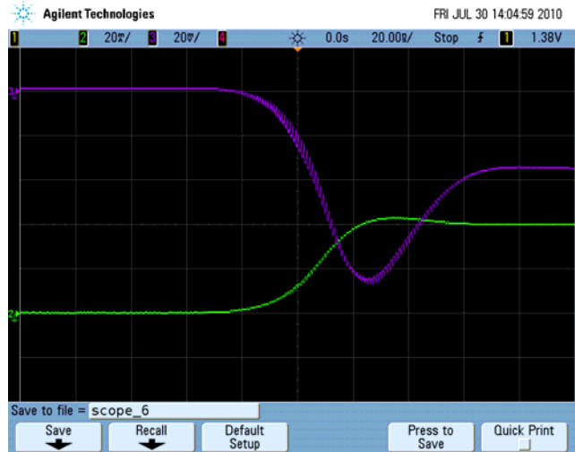
9.6V 700mAh Nicad Transient showing 40mA step with 20nS edge and higher resistance than the Li-Po Battery
