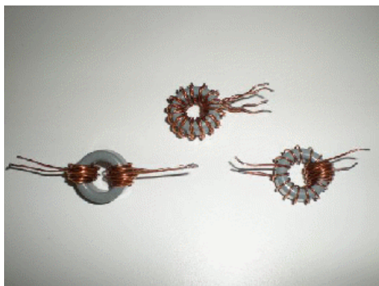
Figure 1. The three transformer samples.
