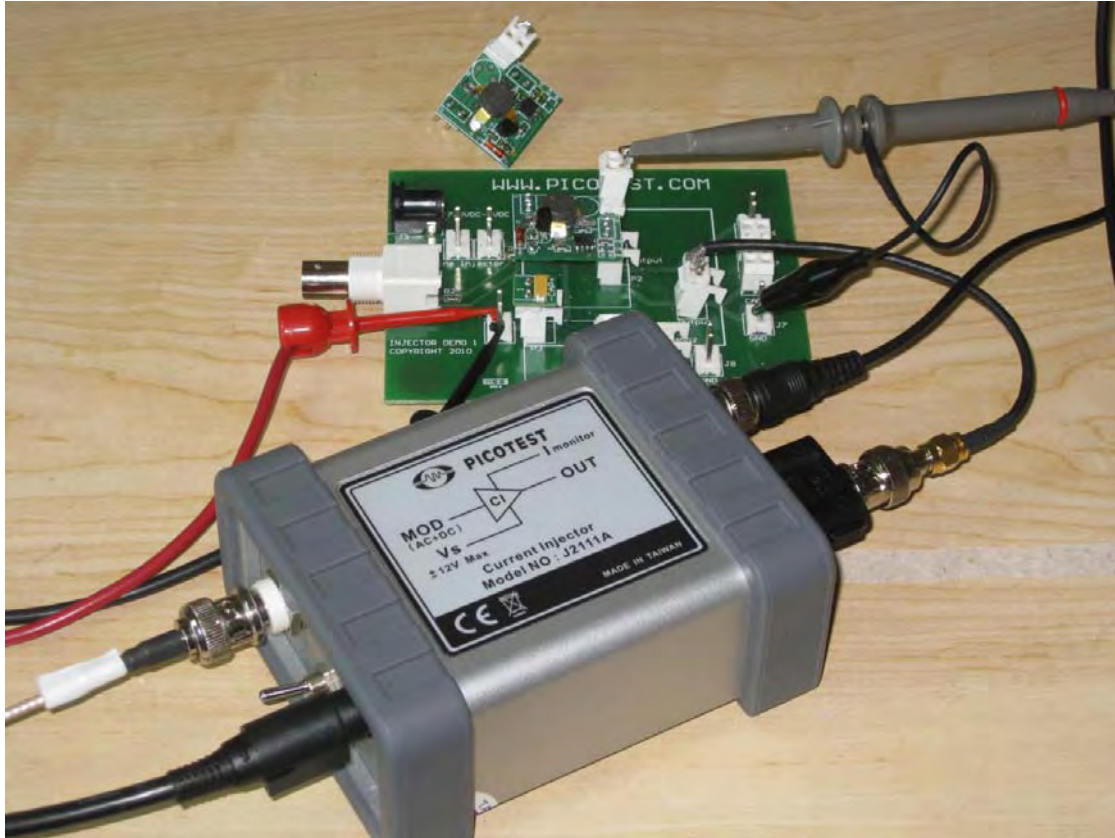
Figure 1 – Impedance test setup for the 300MHz high bandwidth regulator using the Picotest J2111A Current Injector.
