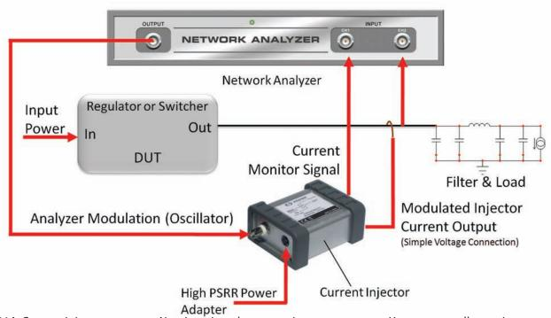
The J2111A Current Injector supports Non-invasive phase margin measurements. You can actually use it to measure the stability of your power supplies WITHOUT having to break the control loop. Simply connect the Current injector output (+ and – leads) to the signal of interest and you can measure the impedance, stability, or step load response.
