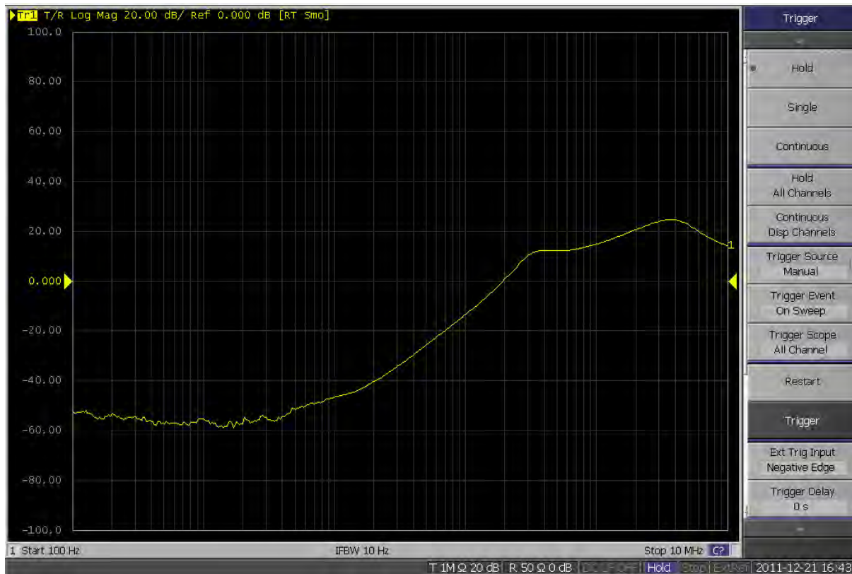
Figure 19 – Crosstalk measurement shown as a voltage gain on the output of the TLV2217 test circuit as a result of current perturbations on the LM317 test circuit.
