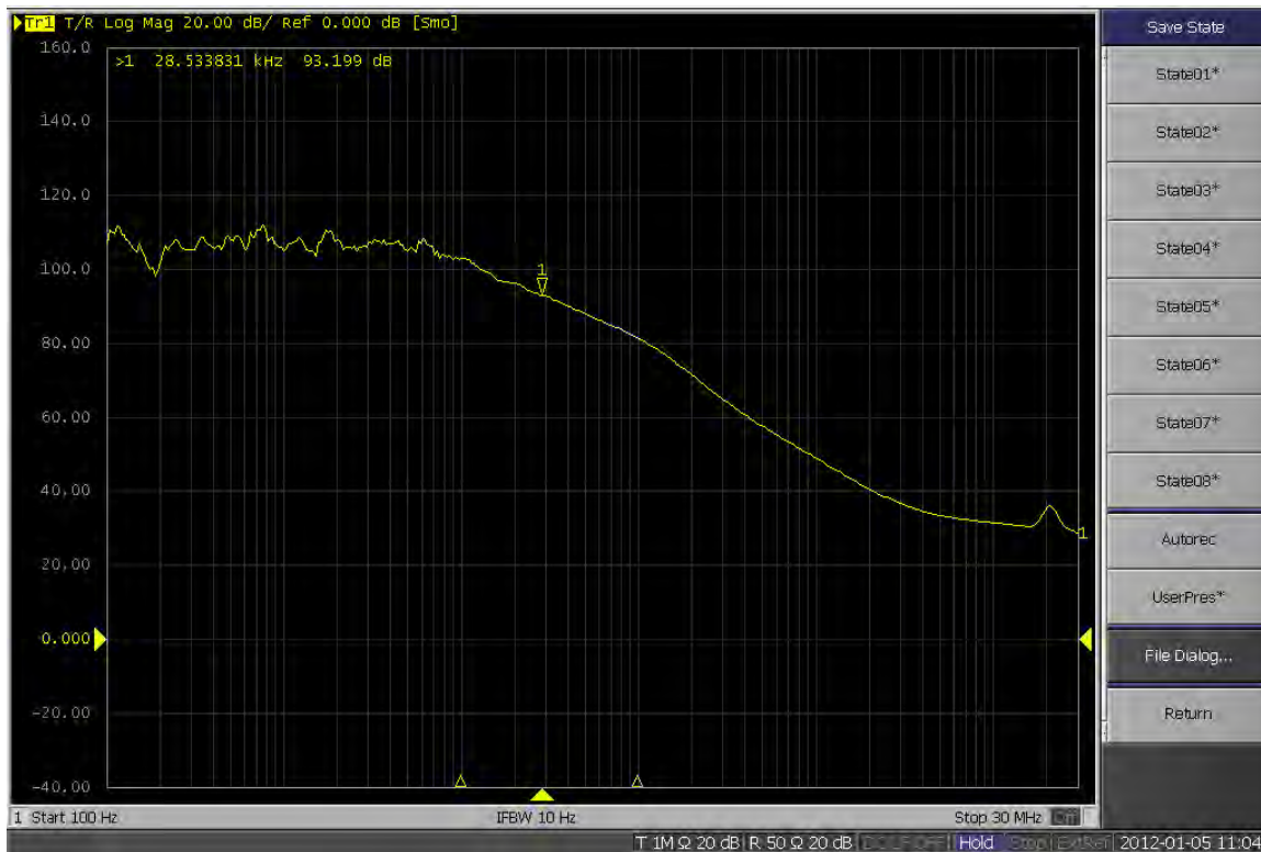
Figure 21 – Input impedance of the LM317 test circuit
