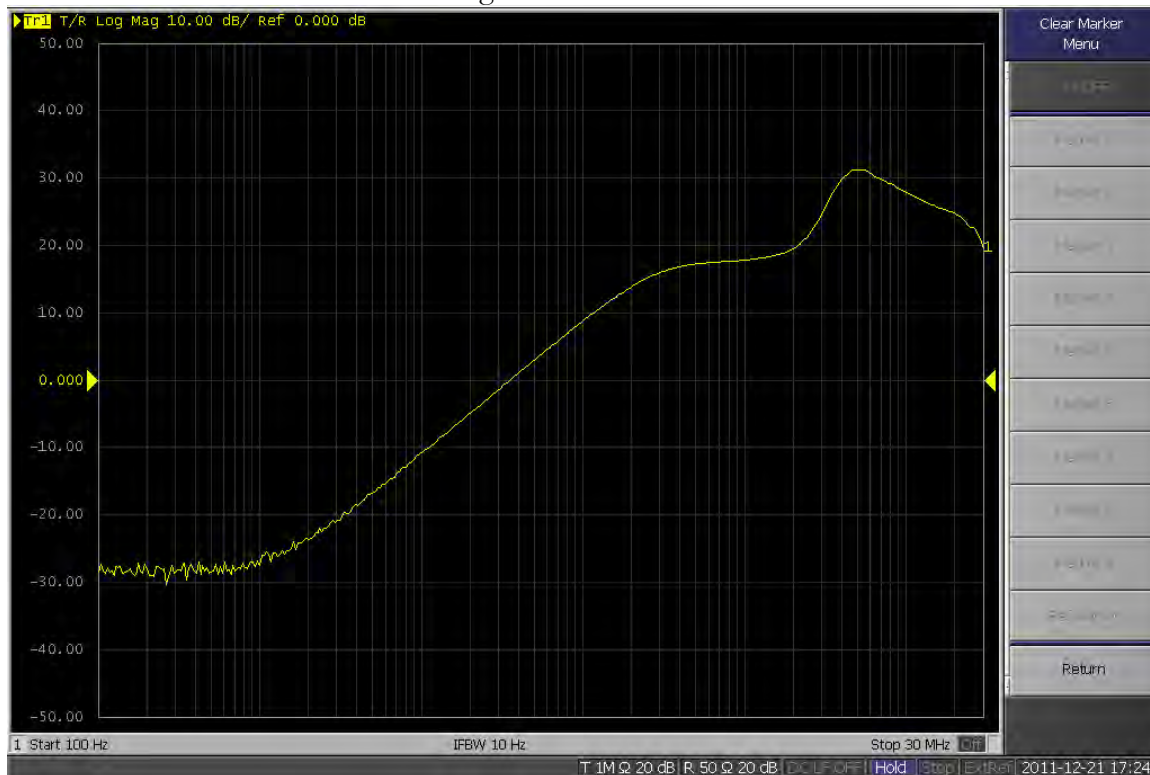
Figure 13 – Output impedance plot of the LM317 test circuit.
